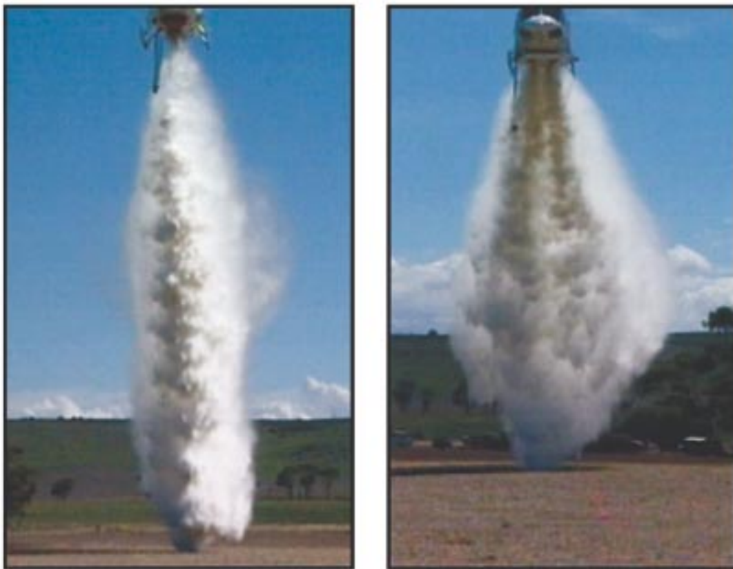
Figure 11 Comparison of the evacuation processes of the Conair (left) and Simplex delivery systems, showing the level of control during delivery
