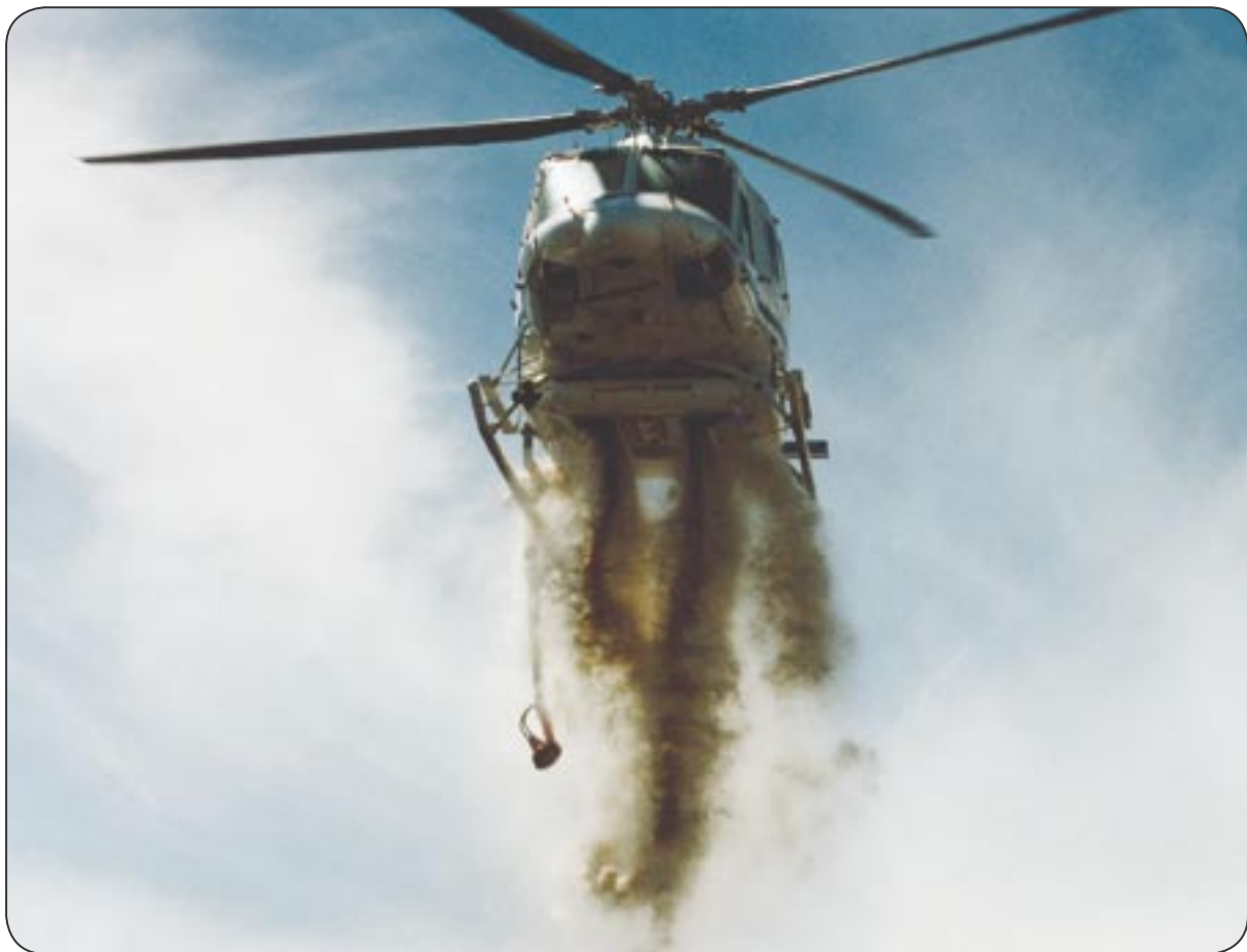
Figure 8 Evacuation of retardant from the Simplex belly-tank showing four clearly-defined flows
