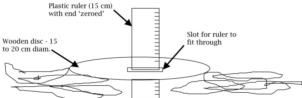
Figure 1.2 Gauge for measuring litter-bed height
