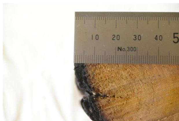
Figure 5: Measuring char depth in a piece of coarse woody debris from a forest ecosystem study area (photograph courtesy Cristina Aponte). Such measurements help to assess changes in pyrogenic carbon stocks due to repeated planned burns.
