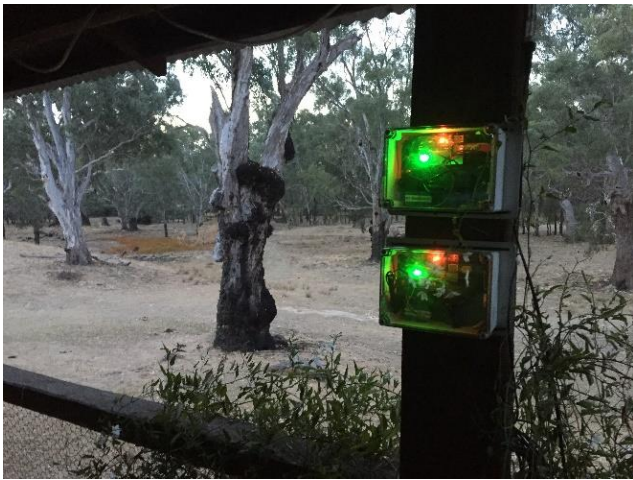
Image 1: Smoke sensors installed at a private property in Gooramadda, Victoria
